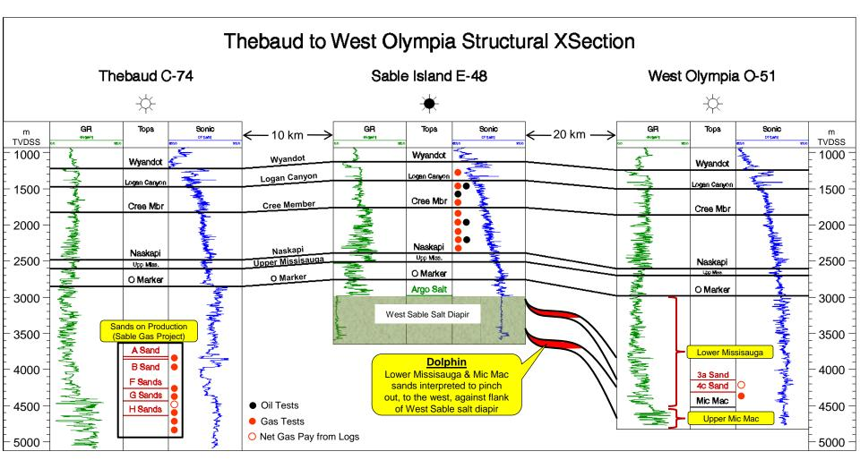
Thebaud to West Olympia Structural Cross-Section. The stratigraphic position of the Dolphin target interval is shown. Note Lower Missisauga and Mic Mac Formation gas sands are shown in red font. The Thebaud gas field is a Commercial Discovery and is currently producing as part of the Sable Gas Project. Sable Island E-48 (West Sable Field) and West Olympia O-51 (West Olympia Field) are both Significant Discoveries. Note this xsection crosses Parcel #2 from southwest to northeast.
